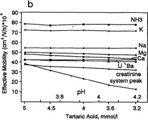
Fig. 1. The influence of 18-crown-6 (a) and tartaric acid (b) on mobilities of cations. BGEs are BGE II (a) and BGE I (b) but with varying amounts of 18-crown-6 and tartaric acid, respectively. All other details are as described in Table 1.
